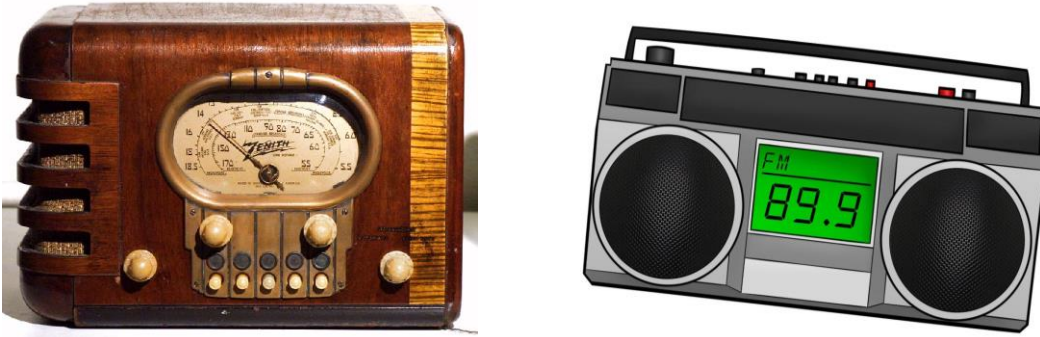
Figure 9: Analog radio (left) allows for tuning to a continuous range of frequencies. Digital display (right) shows only finite discontinuous set of frequencies
