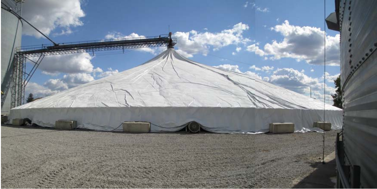
Figure 14: A composite photo of a temporary storage pile at the MAC Marlette, MI facility. A heavy white rubberized-fabric tarpaulin covers the pile. In the center of the photo the circular outlet of one of the suction fans with the tarpaulin draped around it can be seen. Large concrete blocks both hold the side supports for the pile and can also provide ballast to hold the tarpaulin in place. The primary method of securing the tarpaulin is through negative pressure within the pile provided by several fans around the perimeter.
