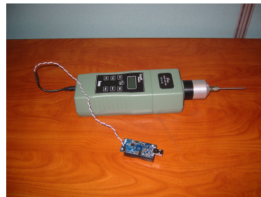
Figure2: Testing set-up with PID-102 (1-Photo-ionization detector and Tmote sky).
