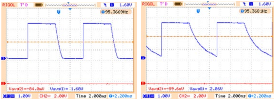
Figure 15. Actual Waveforms: Close object (left) more distant object (right)
