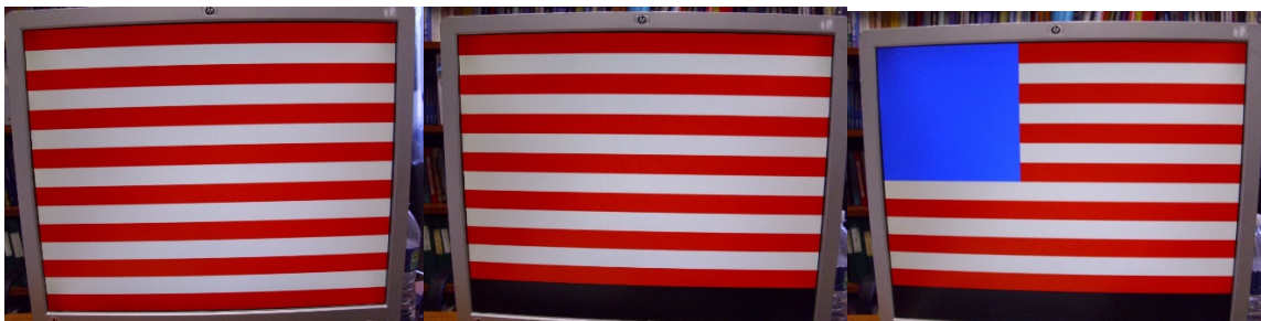
Figure 10. FPGA firmware developed VGA Monitor approximation of an American flag.
