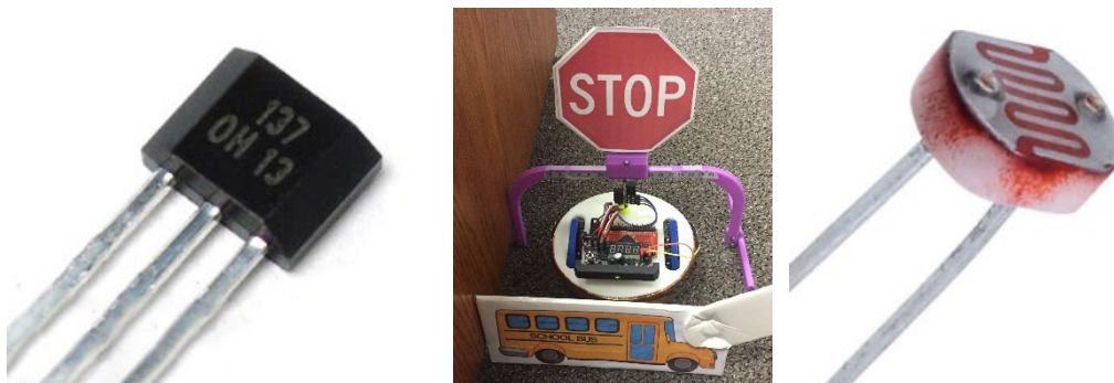
Figure 19. Hall Effect sensor, stop sign, school bus, and CDS Photo resistor.
