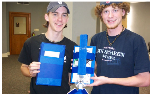
poker chip sorter – uses color sensor
