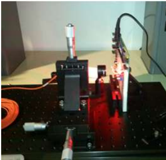
Figure 3: Photograph of the LED, lens system, and multimode fiber with optomechanical mounts and micropositioners.
