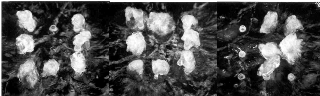
Figure 16 – Viewed from the top, three letters of UOP generated by water jets of microcontrolled fountain. Jets are spaced 2 inches apart. Photos by the author.
