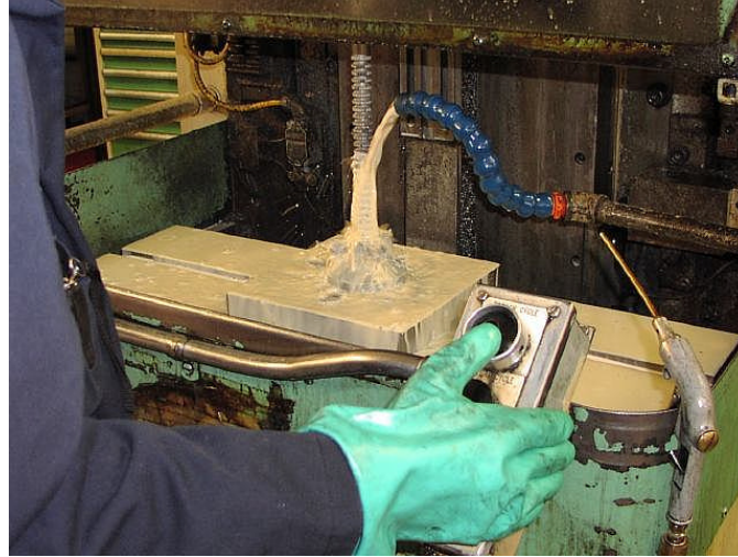
FIGURE 4. Broaching Operation at Focus: HOPE’s Center for Advanced Technologies
