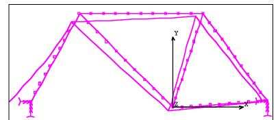
Figure 7 Numerical (FEA) model of bicycle frame in undeformed and deformed states.
