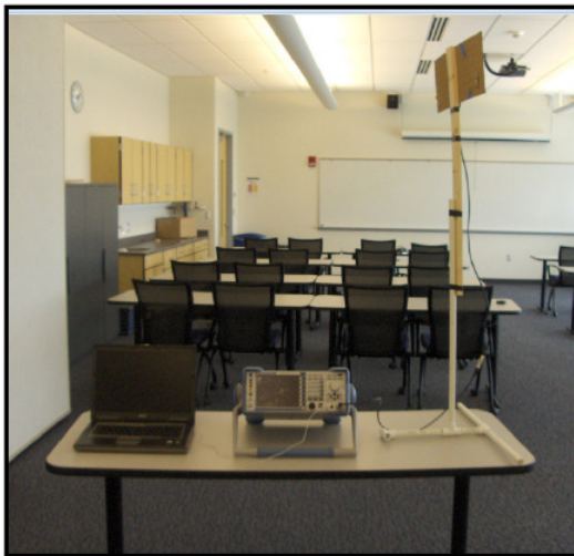
Figure 2: Antenna Radiation Pattern Measurement (left: receiver; right: transmitter)
