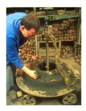
Figure 12: A stickle is used in the process of creating a bell. A stickle smoothes the inner and outer surface of a bell<sup>27</sup>.
