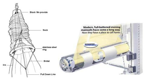
Figure 13: Two solutions for dousing a sail<sup>28</sup>.
