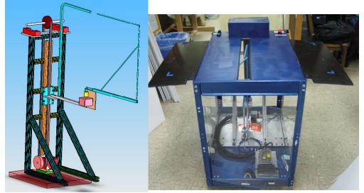
Figure 11: Original team's award winning solution to the laundry folding problem. The image on the right shows the final solution and the left image is the internal mechanism. The towel or wash cloth is spread out on the top surface of the device. A bar rises in the center causing the item to fold in half. Half of the bar rotates around causing another half fold in the towel.
