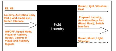
Figure 5: Black box model for the laundry folding device.
