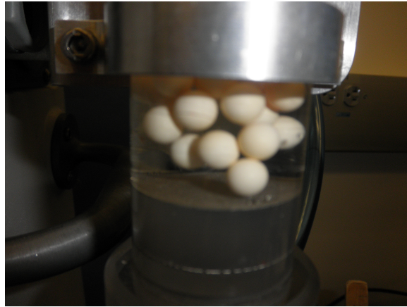
Figure 3. Separation of large beige particles towards the end of the elutriator despite the presence of more dense, but tiny glass beads.
