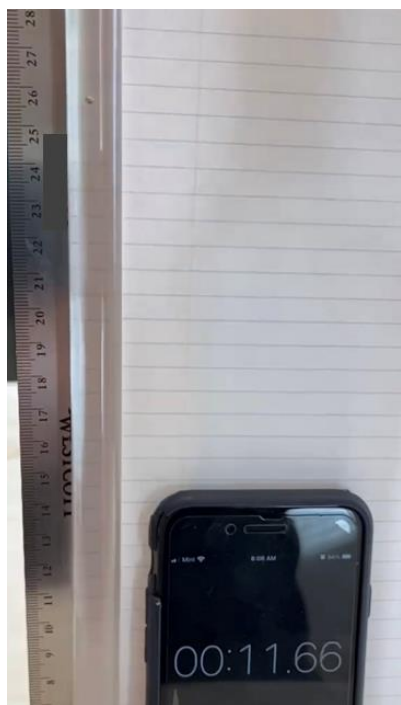
Figure 1: Trial run with a 2 mm ball bearing and a ½” tube
