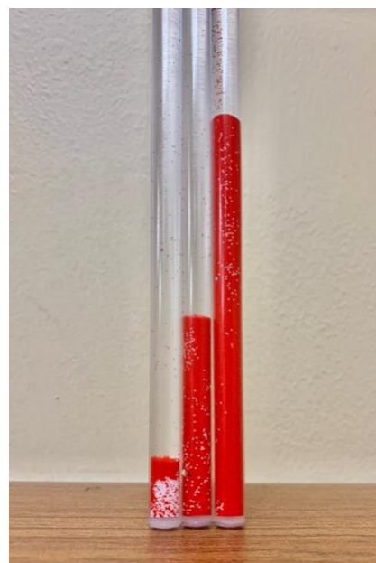
Figure 1. Cell settling device prototype that demonstrates hindered settling as bead population density increases
