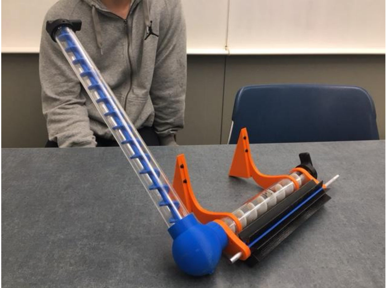
Figure 6 The final fabricated Archimedes screw and paddle design to pick up objects.
