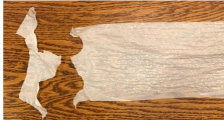
Figure 4: Member with fracture in the net section
